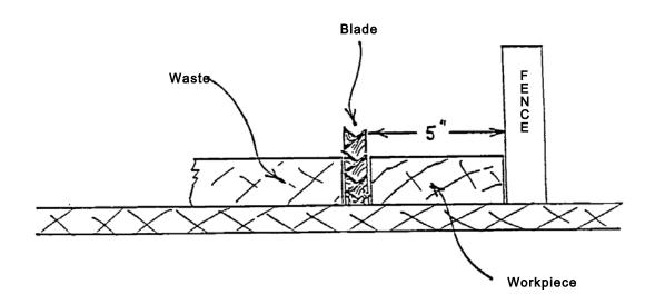
Set the fence to cut 21-3/4" width. Check to see if the fence is parallel by measuring from teeth at the front and rear of the blade. The measurements should be equal. Check with instructor if the fence is not parallel. See sketch.
