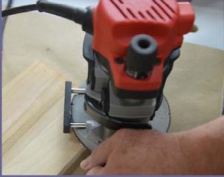
Only 25% of the router base is supported at the corner.
