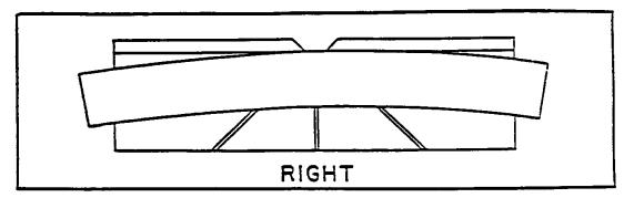
When cutting flat pieces, first check to see if the material is bowed. If it is, make sure the material is positioned on the table as pictured above.
