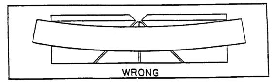
If the material is positioned the wrong way, as shown above, the material will pinch the blade near the completion of the cut.
