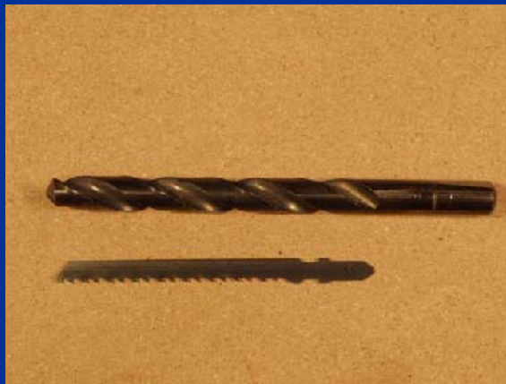
Drill holes larger than the saw blade.
