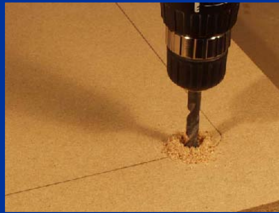
Drill holes near the corners
