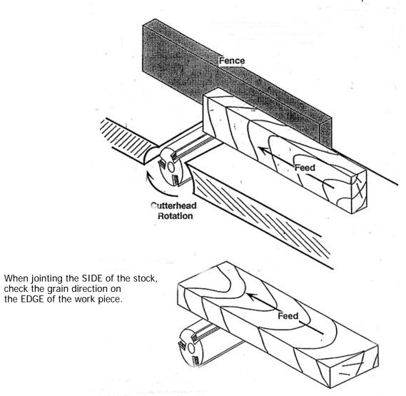
NOTE: When the cutter head is below the stock, as on the jointer, the knives will *exit* the stock <u>toward your feet</u>. The wood grain should be oriented in the same general direction
